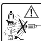
**CAUTION.** pressure cleaners can be dangerous if they are not operated correctly! The jet must never be directed at people, animals, electric equipment connected to the power supply or against the actual pressure cleaner.
